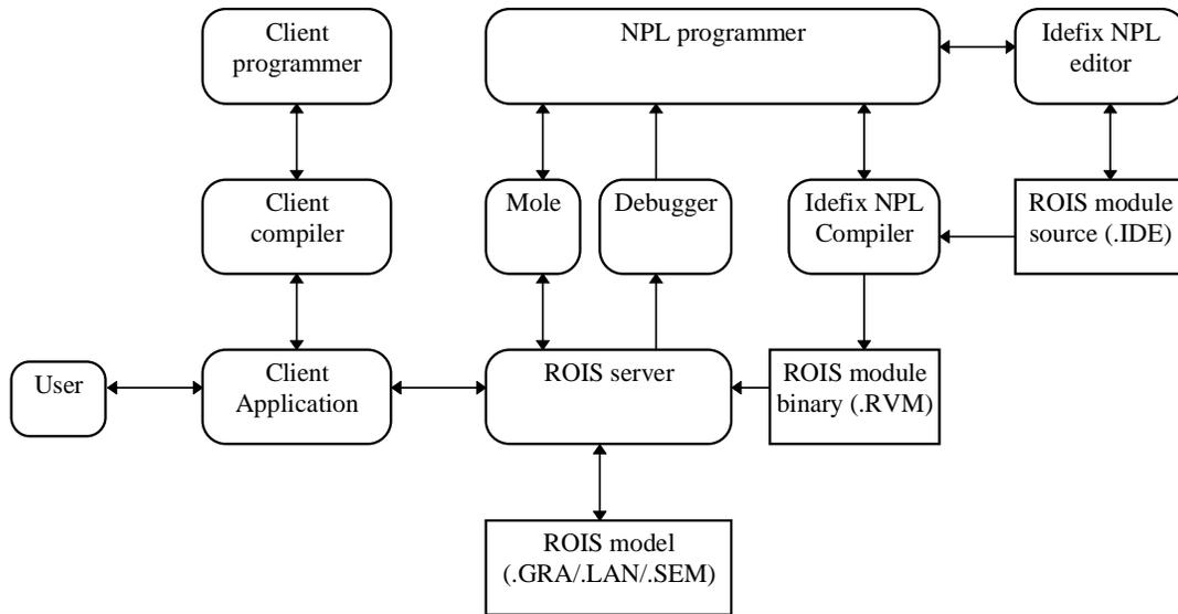
figure 18: Data flow diagram of ROIS system development process.
